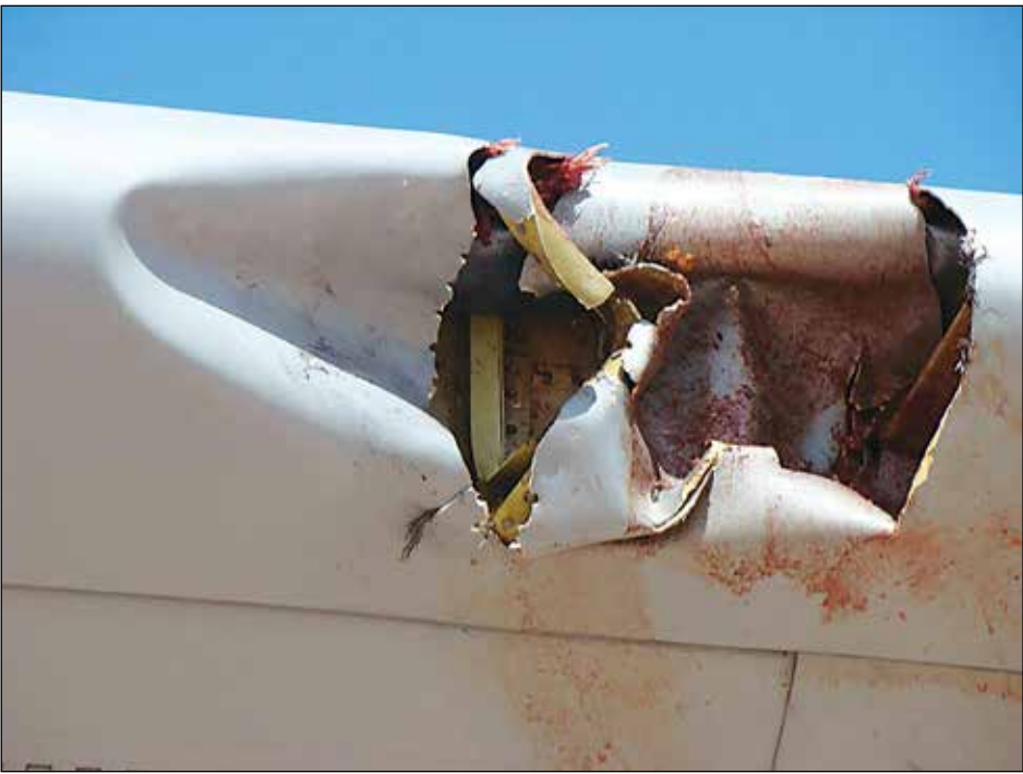
Courtesy of 97th AMW Wing Safety Division This illustrates the damage a bird can cause on the wing of an airplane.
