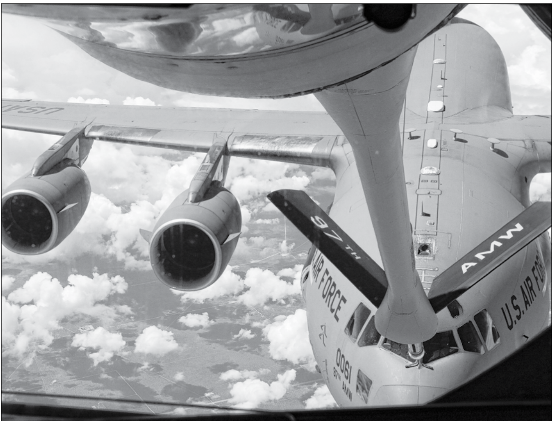
Katrina Goforth | Altus Times From the boom of a KC-135, the boom operator makes contact for air refueling with a C-17 over southwest Oklahoma. The 97th Air Mobility Wing at Altus AFB specializes in training pilots in both aircraft.
