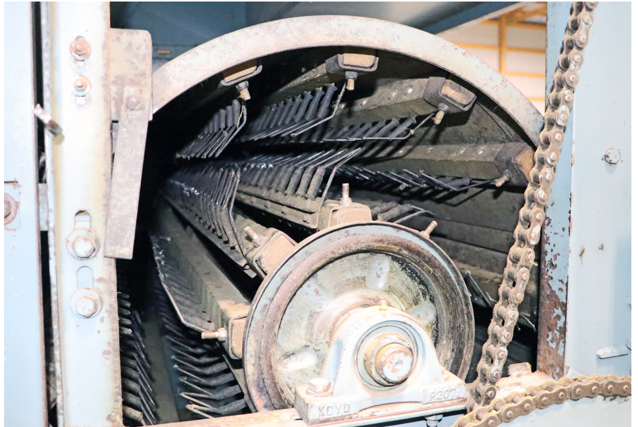
The Wolf WHE 280 hop harvester separates the hop cones from the plant itself.
